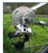
(Above) Correctly sized cranks! (Below) An 11-34T 8-speed cassette gives a wide, user-friendly gear range
